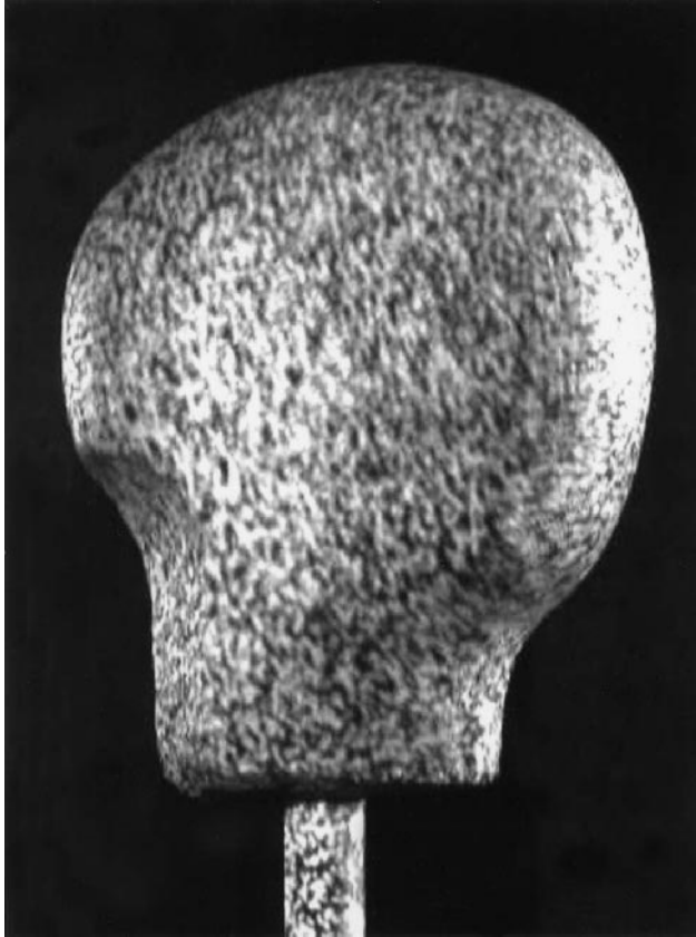
Fig 3 Random infrared pattern projected onto the surface.
