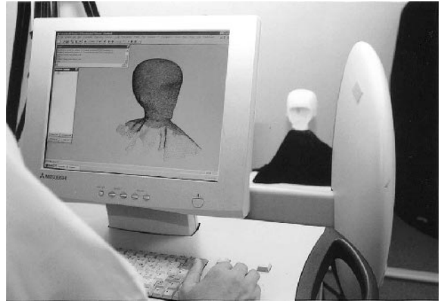
Fig 8 Image of plaster model on screen as model is being digitized.
